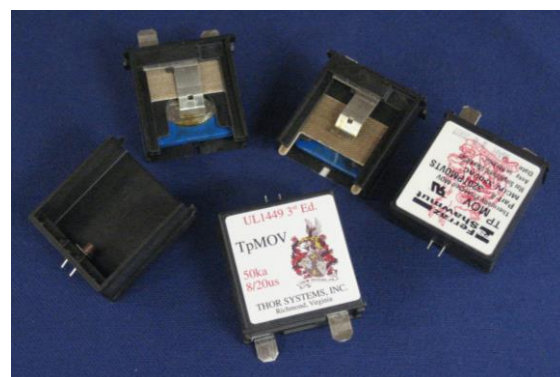
Thermally Protected Metal Oxide Varistor (TpMOV) "Fail-Safe Device"
